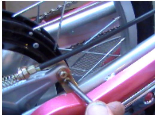
Loosen the brake bracket on the frame and remove the other bolt that holds the brake arm.
