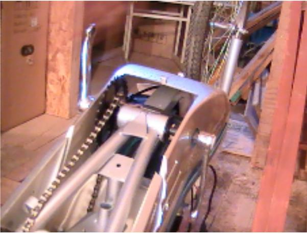
Now lift the wheel assembly out **watching the placement of the washers and brake apparatus**
